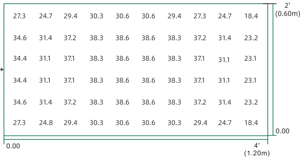
This map displays PAR distribution in an area of 4'x2'(1.2mx0.6m). The distance between the lights and the plants is 0.98'(0.30m), and 2pcs 315-0007 are needed in the planting area of 4'x2'(1.2mx0.6m).
